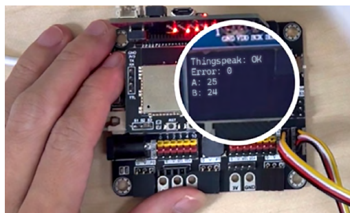
LCD screen showing ThingSpeak connection status and distance measured by the ultrasonic sensors
